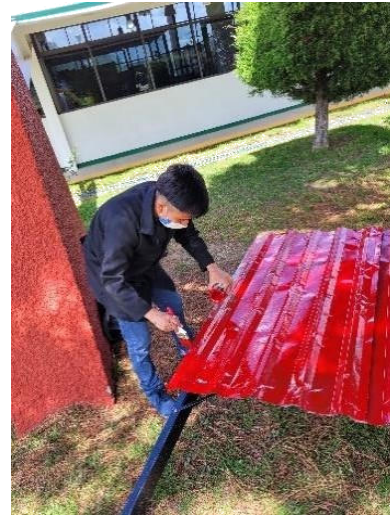
FIGURE 12: Hydroponic system paint coating. Source: Own, year 2022.
